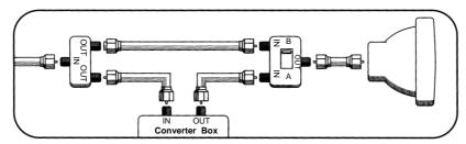
When the A/B switch is in the A position, you need to change channels on the converter box (and your TV should be tuned to channel 3 or 4); when the A/B switch is in the B position you can change channels on the TV.
